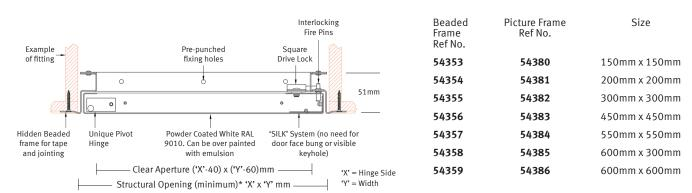
**Door Tray & Frame:** Formed from 1.0mm and 1.2mm Zintec electrogalvanised mild steel with a 25mm wide frame either perforated or solid finished in polyester powder coat white RAL 9010 20% Gloss.
