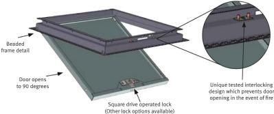
Fire Rated Access Panels provide fire rated protected openings in ceilings and walls for access to building engineering services. Available fire rated up to 2 hours, the doors are finished in powder coated white and can be over painted to blend with the surrounding surface.
