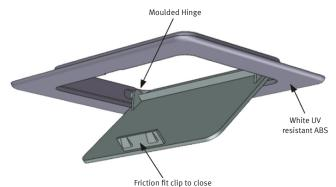
Plastic Access Panels provide a high quality low cost solution for access to building services in ceilings and walls. Primarily used in domestic situations for access to rodding eyes and stop cocks the panels are very simple to fit.
