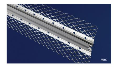
Protektor Movement Bead provides a solution to thermal movement in plaster and rendered finishes.
