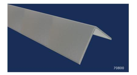
Protektor Corner Guards are easily installed over 90° finished corners and provide a high level of impact corner protection on plasterboard partitions and also retro fitted to existing constructions. Available in a variety of sizes ranging from 25mm x 25mm, 38mm x 38mm and 50mm x 50mm.
